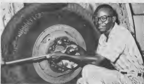
A METHOD to adjust brakes without removing the brake drums of fork-lift trucks was suggested by J. Warner. The idea earned Fls. 35. UN METODO pa ajusta brake sin kita e drum di wiel di trucknan cu forklift a wordo sugeri door di J. Warner. E idea a gana Fls. 35.
